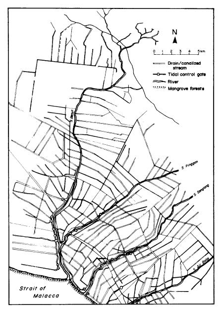
Fig. 2. Drainage controls in Sg. Benut catchment.
